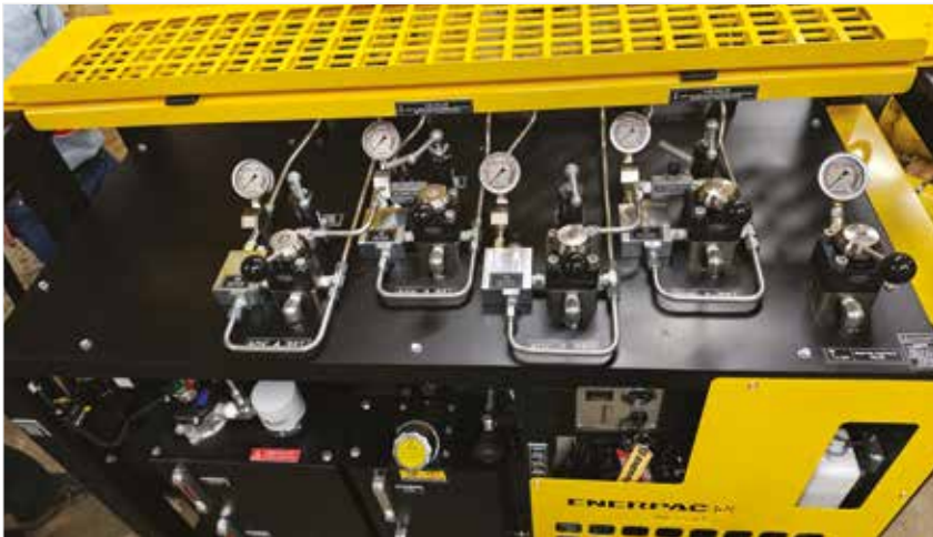
▲ 4-way, 3-position manual control valves for Advance/Hold/Retract of single or double-acting cylinders. Adjustable pressure relief valve and pressure gauges per circuit.
